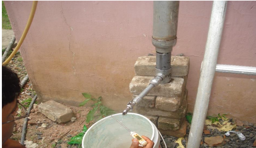
Fig 6.7. The flow of Condensate as a result of Steam Condensation Heat Balance, considering a typical reading,
