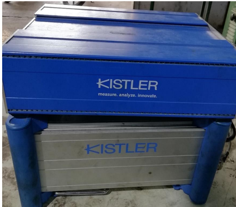
Figure 3.10 :Cutting force -charge amplifier &Data acquisition system
