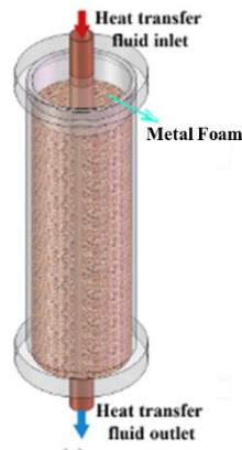
Fig. 2.5 Shell and tube heat exchanger with metal foam [121]
