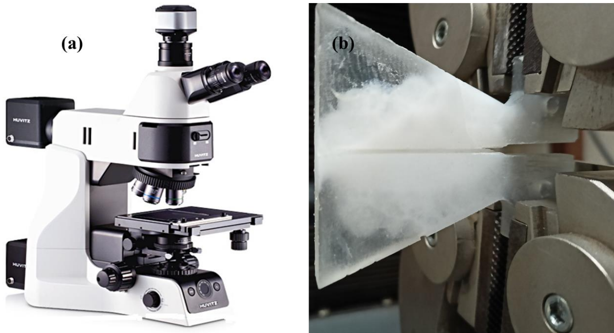
Figure 4.4 (a) Huvitz 3D optical microscope (b) TDCB specimen during mode I fracture test
