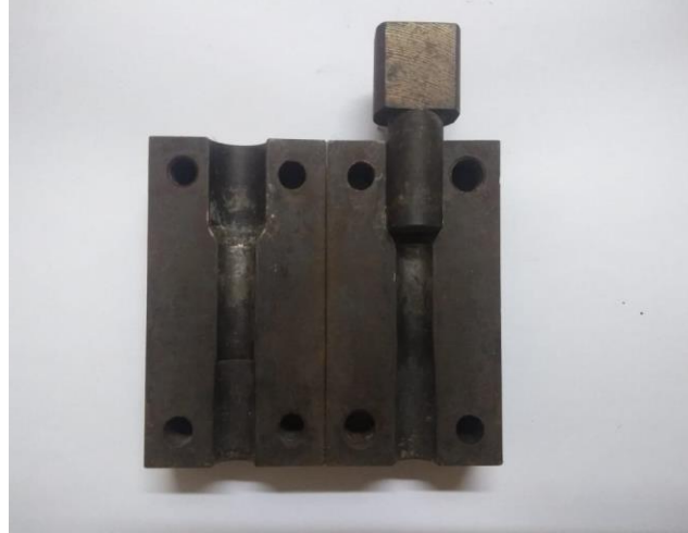
Fig 3.8: Extrusion die of ratio 4 and approach angle 60^\circ with plunger
