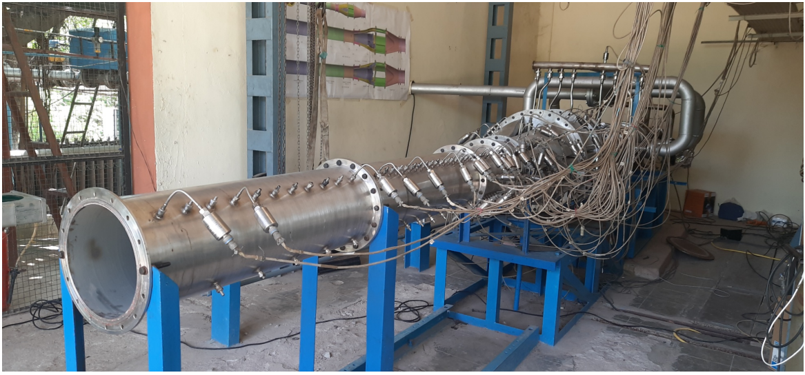
Figure 3-68 DCR Engine mounted on test bed with instrumentation
