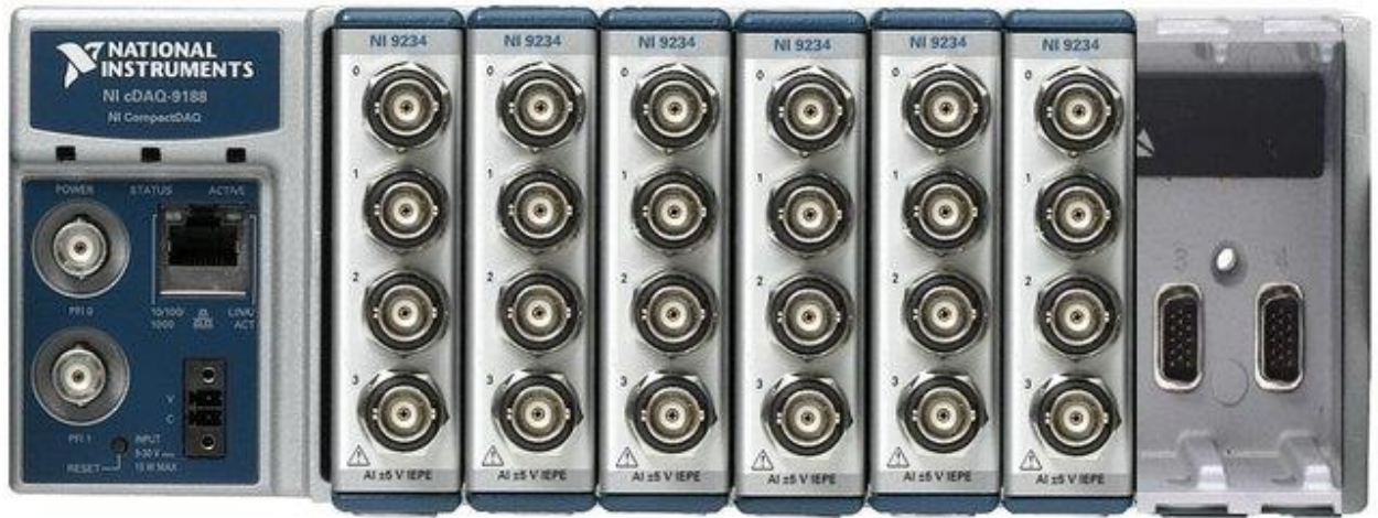
Figure 2.4 A typical multi-channelled data acquisition system
