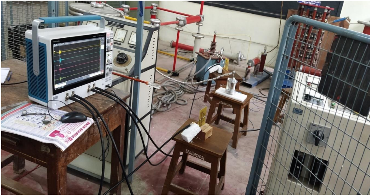
Figure 5.23 Laboratory Experiment Model for PD source Localization using Broad band LPDA UHF sensors
