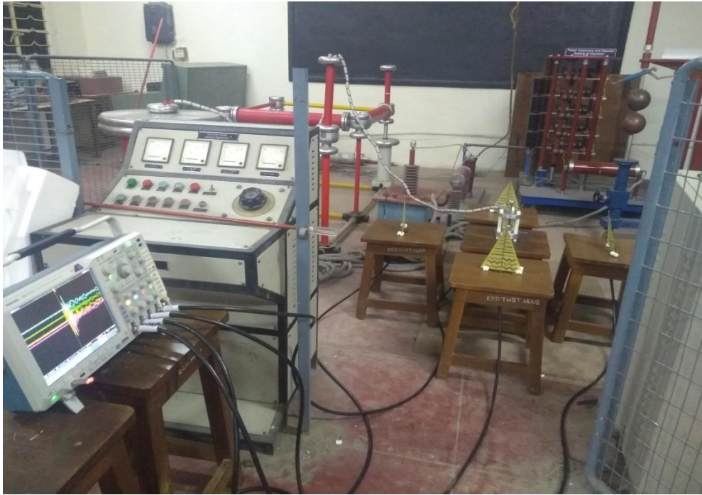
Figure 5.19 Experiment Model for localization of PD source position number 1 in table 5.5
