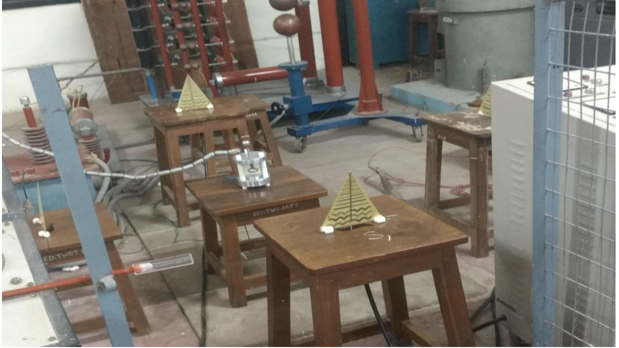
Figure 5.21 Experiment Model for localization of PD source position number 2 in table 5.5
