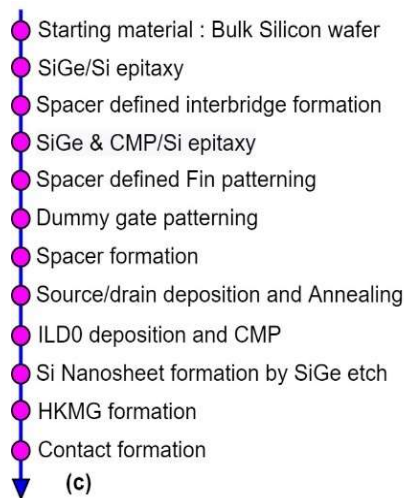
Fig. 6.2: Process Flow of CombFET [75], [135].
