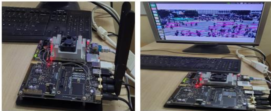
Figure 6.5 Experimental setup and captured results on Jetson Tx2 Evaluation board.
