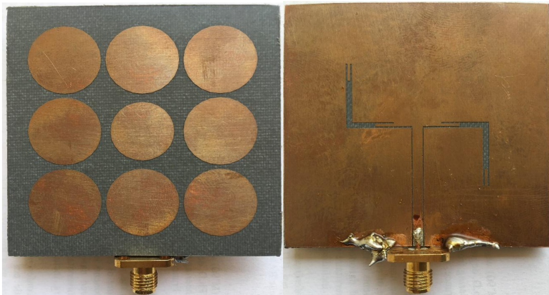
Fig.4.19. Fabricated prototype of proposed antenna (a) top plane view (b) bottom plane view
