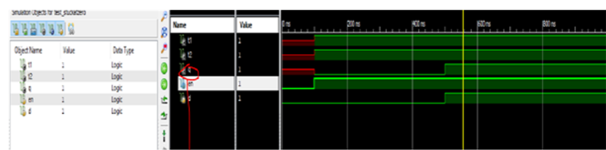
Figure 4.18 Stuck at ‘1’ operation of DFF
