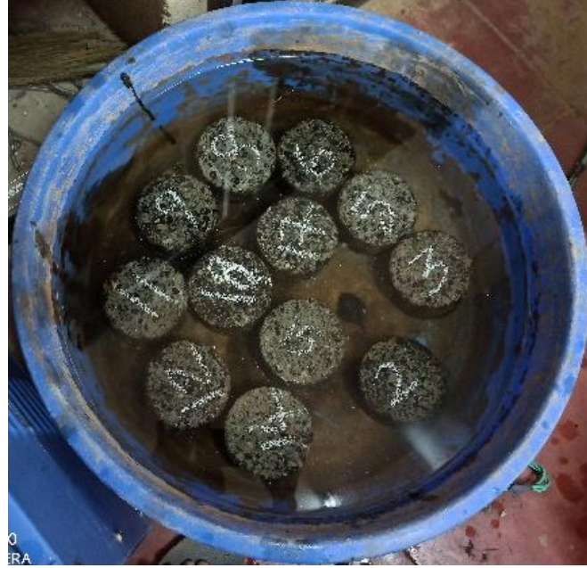
Figure 3.9 Conditioning of samples underwater
