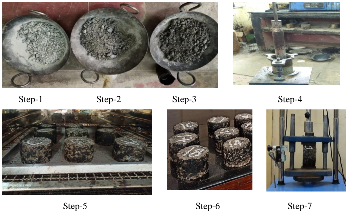
Figure 3.7 Steps involved in the mix design of EATB
