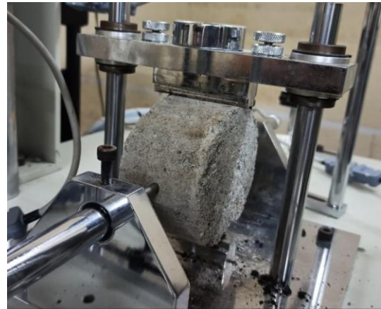
(b) Setup to measure deformation
