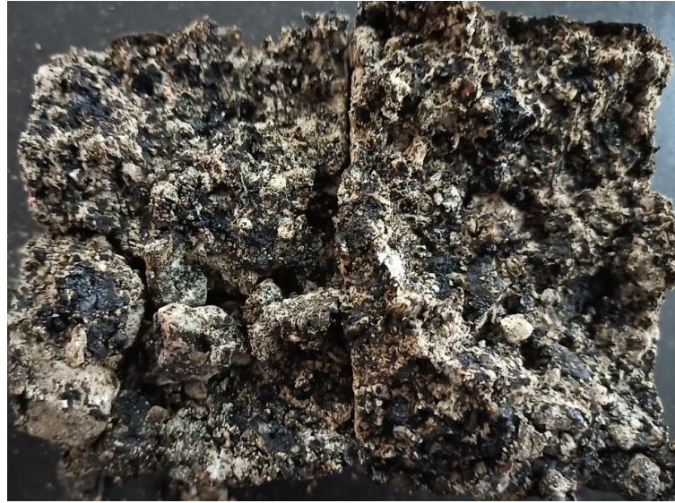
Figure 5.9 Failure patterns of RAP blends
