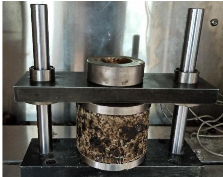
Figure 3.11 Dynamic creep rutting test apparatus
