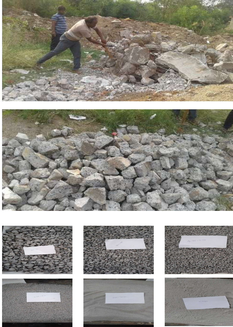
Figure 3.1 Processing of concrete waste to obtain RCA.
