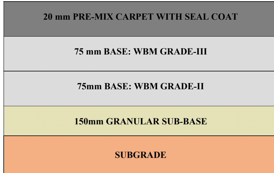
Figure 1.2. Typical cross-section of LVRs
