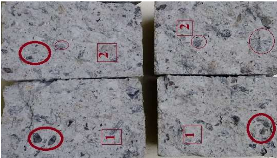
Figure 5.2. Failure of the specimen after fatigue test.
