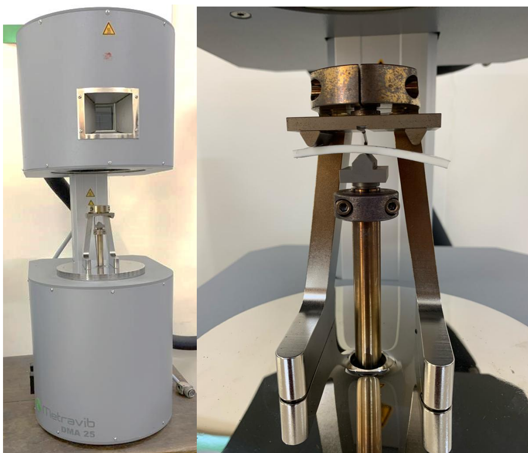
Figure 8.2: Experimental set-up for DMA testing
