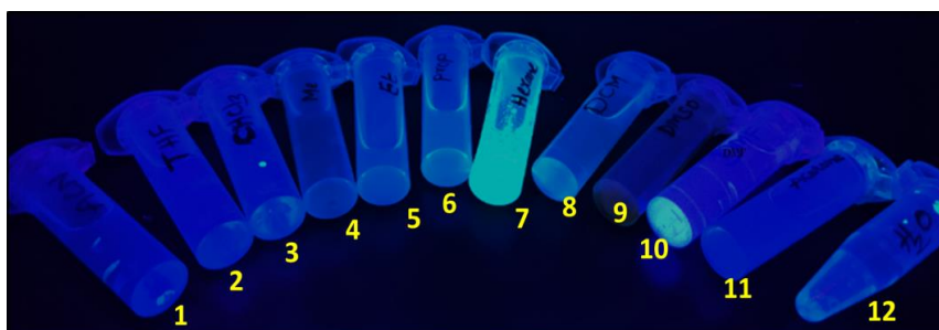
Figure 5A.9 Visual fluorescence picture of 3FMC-2AB-OEt in acetonitrile (1), tetrahydrofuran (2), chloroform (3), methanol (4), ethanol (5), propanol (6), n-hexane (7), dichloromethane (8), dimethylsulphoxide (9), dimethylformamide (10), acetone (11) and water (12)
