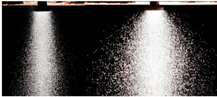
Figure 2.4: Variation in the flow pattern of atomization with change in power of atomization (a) 3 W and (b) 9 W Ramisetty et al. (2013).
