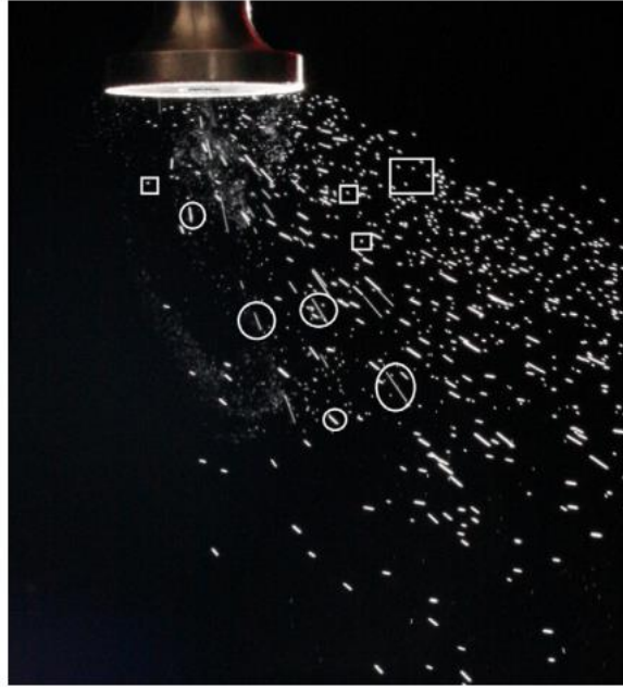
Figure 2.3: Droplets ejection at high velocity streaks caused due to the cavitation effect. Streaks are depicted in circles and droplets are depicted in squares Ramisetty et al. (2013).
