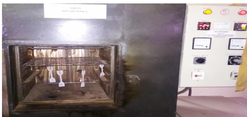
Figure-59: Hot air oven ageing in progress at 90°C
