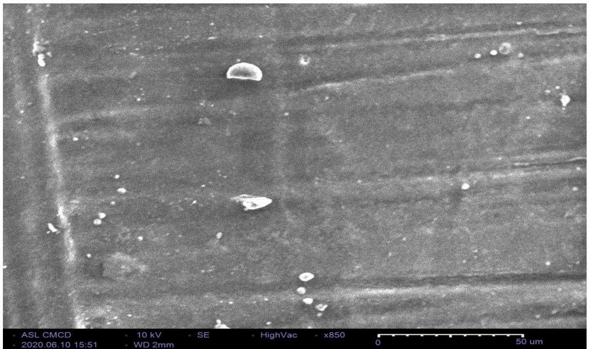
Figure-55: SEM image of Nitrile Rubber based insulation
