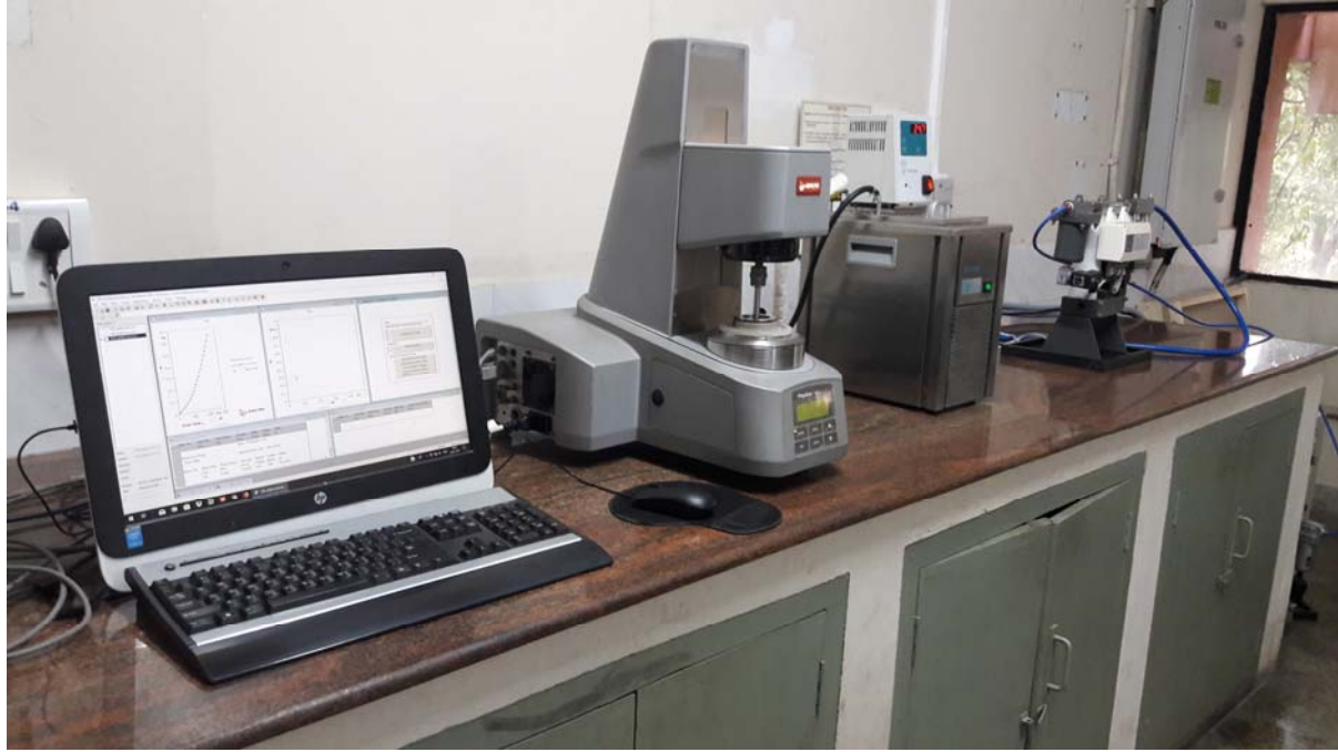
Figure 5. Experimental setup of Anton Paar Physica MCR101 Rheometer
