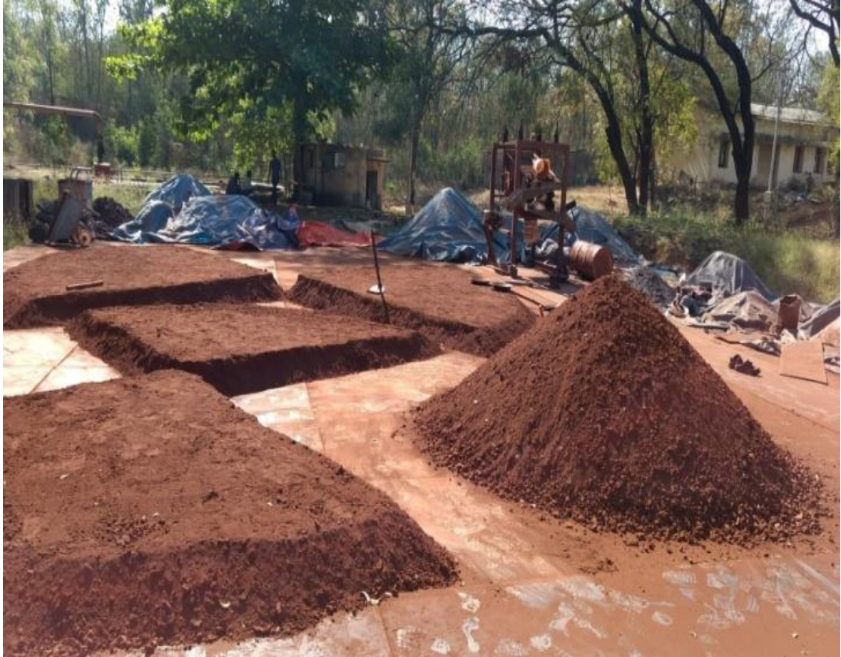
Fig.3.2 Sampling and sample preparation by coning and quartering process
