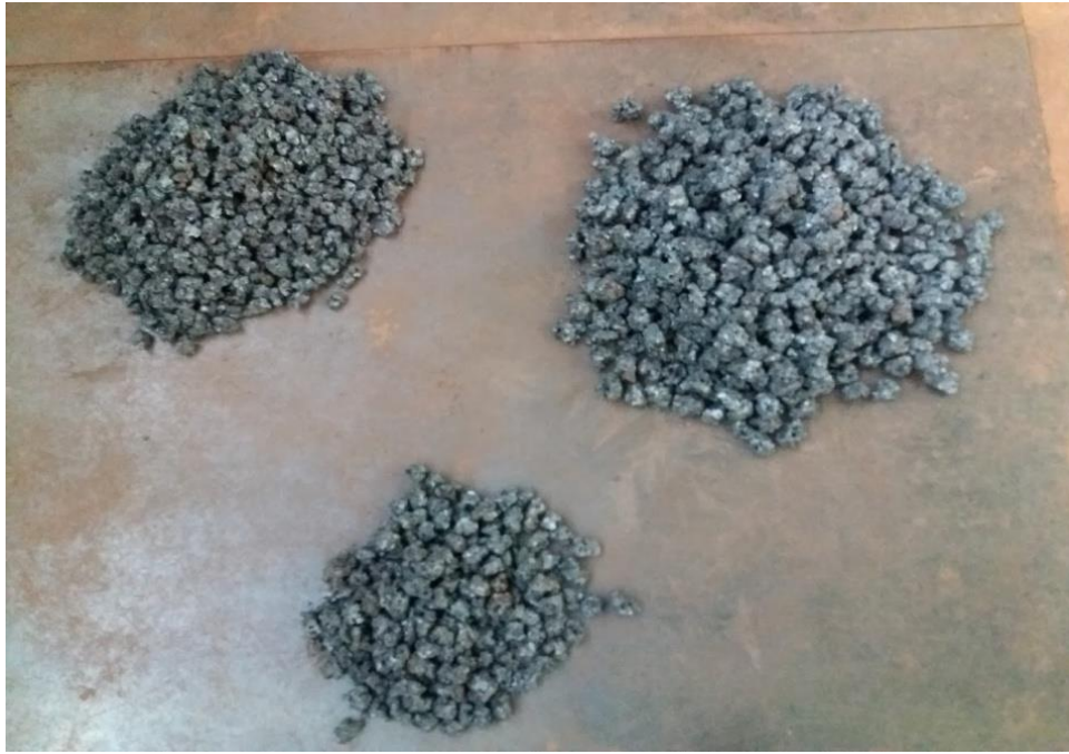
Fig.3.22 Sizing and sampling of sinter prepared in pot grate furnace
