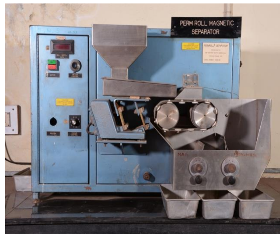
Fig.3.13 Permroll magnetic separator (STEARNS Roll)
