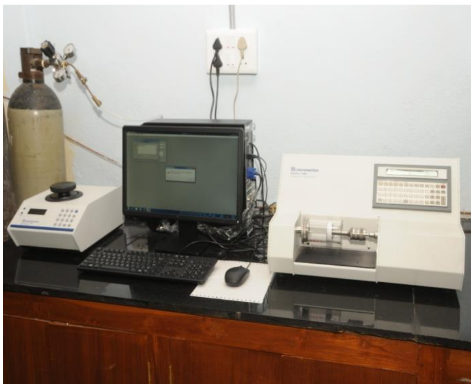
Fig.3.3 Gas pycnometer (AccuPyc 1340)
