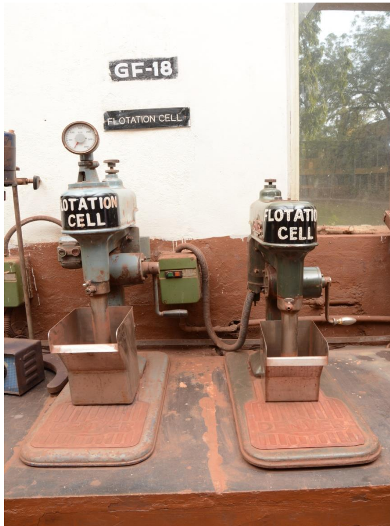
Fig.3.14 Denver laboratory scale flotation cell
