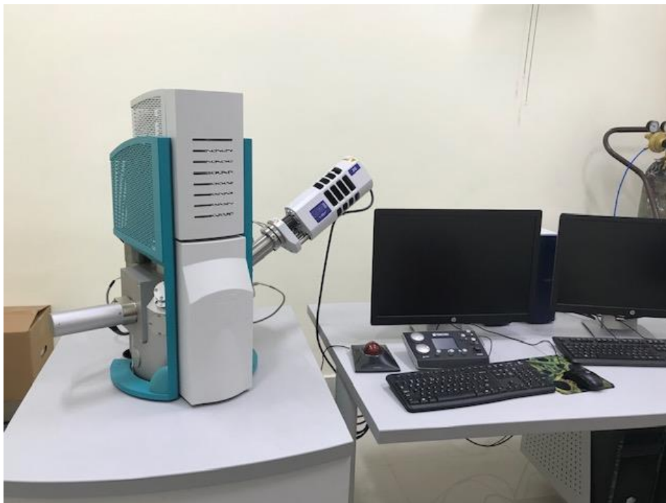
Fig.3.8 Scanning electron microscope (make: TESCAN)
