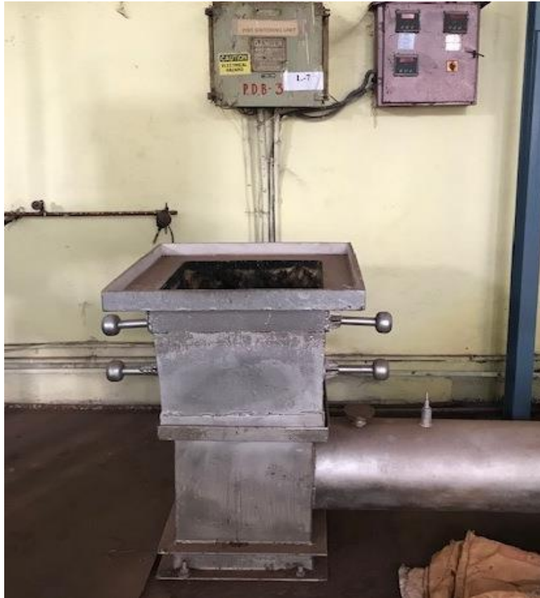
Fig.3.20 Pot grate furnace for sintering
