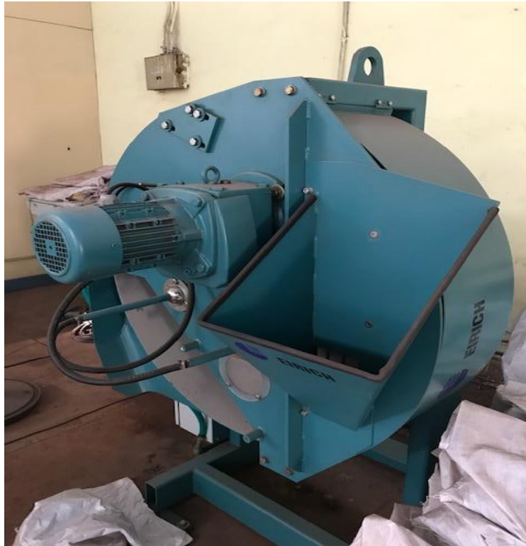
Fig.3.18 Eirich make disc mixer
