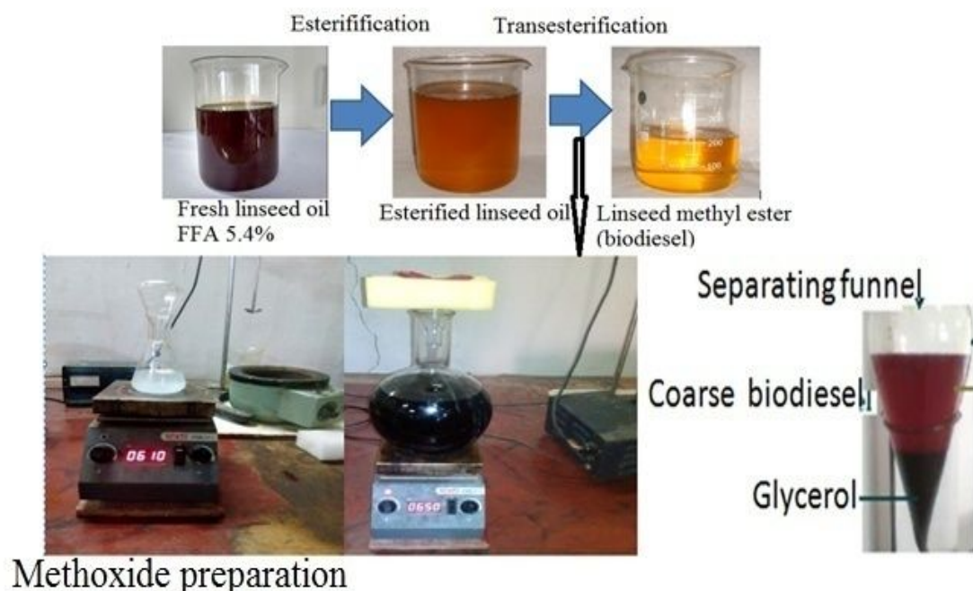
Fig. 3.4 Stages of biodiesel preparation in the laboratory
