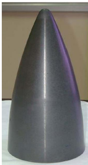
Figure 1. 2. Image of sintered and machined \beta -SiAlON radome (Ganesh, 2011)
