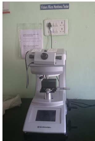
Figure 3.16: Micro Vicker's hardness tester (Make: Shimadzu, Model: HMV-G20ST)
