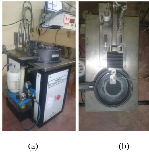
Figure 3.19: (a) Snapshot of two body abrasive wear testing of sample (b) Top view of abrasive wear testing of sample
