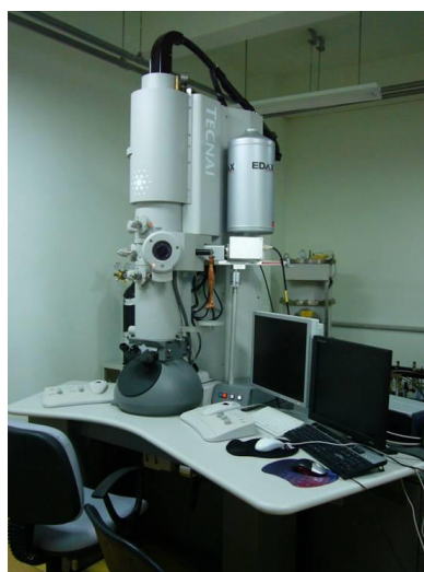
Figure 3.12: Transmission electron microscopy equipment at Hyderabad Central University
