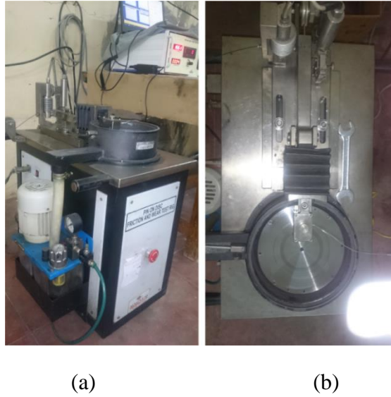
Figure 3.17: (a) snapshot of dry sliding wear test of sample (b) top view of dry sliding wear test of sample
