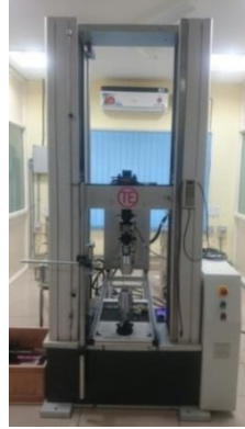
Figure 3.13: Electro-mechanical universal testing machine (Blue Star WDW-100S) at NIT Warangal
