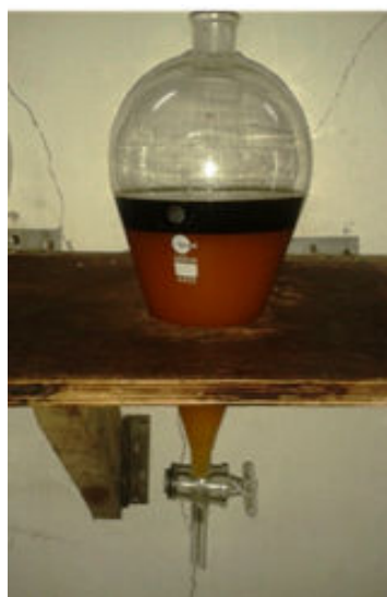
Figure 3.9 Settled Karanja esters in a separating funnel
