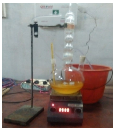
Figure 3.4 Reactor for biodiesel conversion
