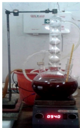
Figure 3.8 Esterification of Karanja oil in a reactor
