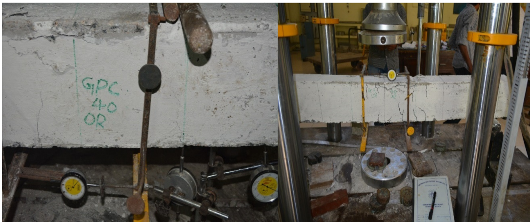
Figure 6.10: Crack pattern of GPC 20 MPa
