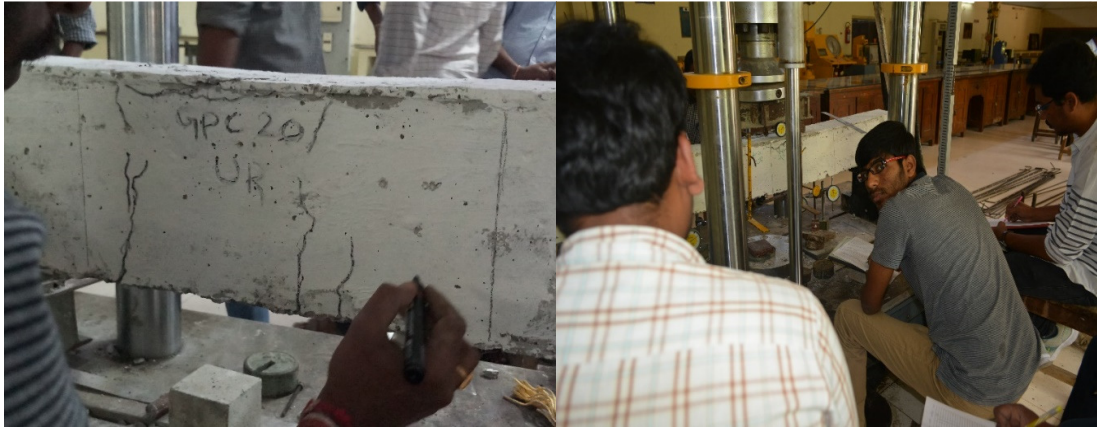
Figure 6.10: Crack pattern of GPC 20 MPa
