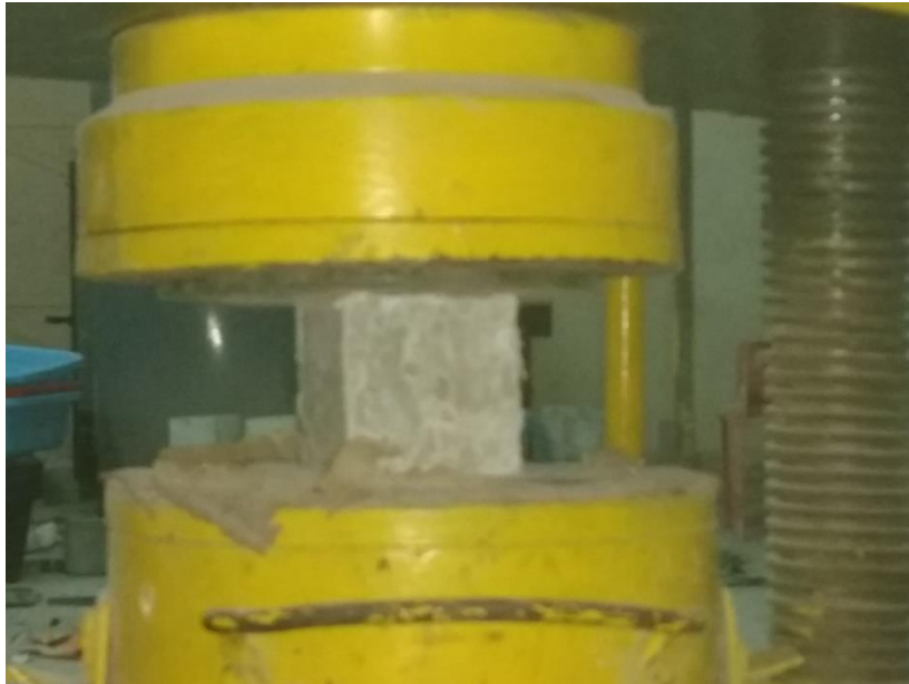
Fig.4.6 Testing of cube under compression
