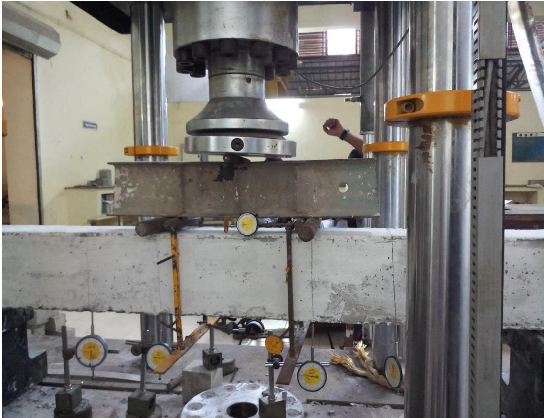
Figure 6.6: Test setup for Moment curvature values
