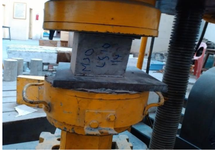
Figure 4.3: Testing of cube under direct compression
