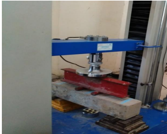
Figure 4.5: Testing of prism under flexure
