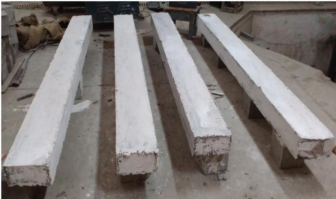
Figure 6.5: Beams ready for experimental moment curvature testing
