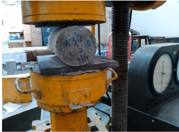
Figure 4.4: Testing of cylinder for split tensile strength
