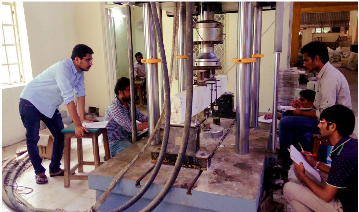
Figure 6.7: Experimentation on the beam for moment curvature relationship
