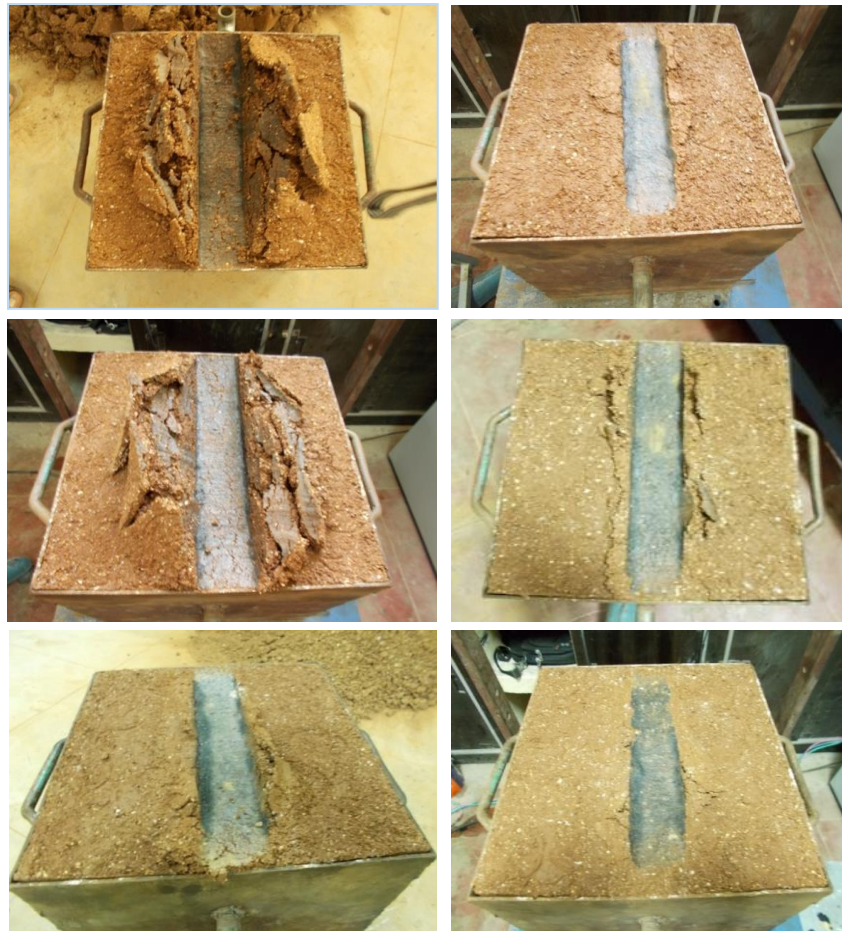
Figure 27 Snapshots of without and with reinforcement of coir geotextile
