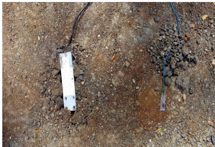
Figure 3.16 Installation of load cells and strain gauge into the subgrade
