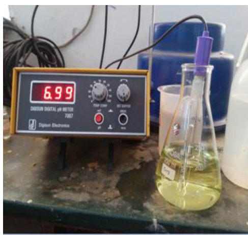
Fig 3.8 pH stabilization of influent heavy metal solution
