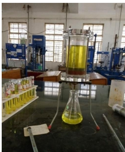
Fig 3.9 Column Experiment with heavy metal as influent solution
