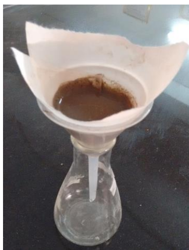
Fig. 3.5 Filtration of Sample using Whatman filter paper no.42
