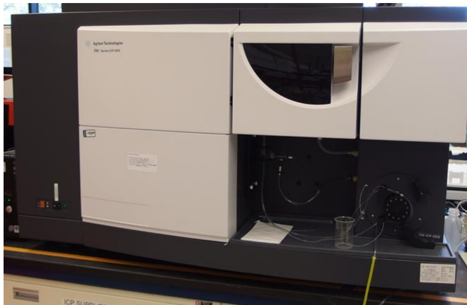
Fig. 3.6 ICP-OES instrument for checking metal concentration in the effluent
