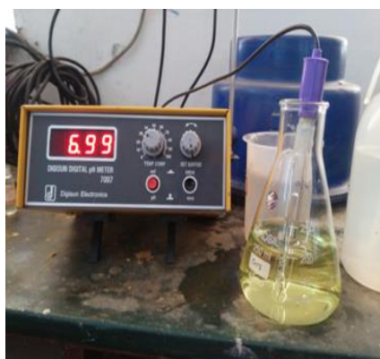
Fig. 3.3 pH stabilization of soil solution matrix
