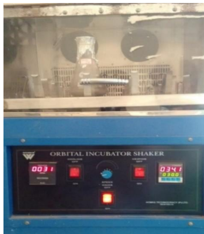
Fig. 3.4 Soil solution matrix under agitation in Orbital Incubator Shaker
