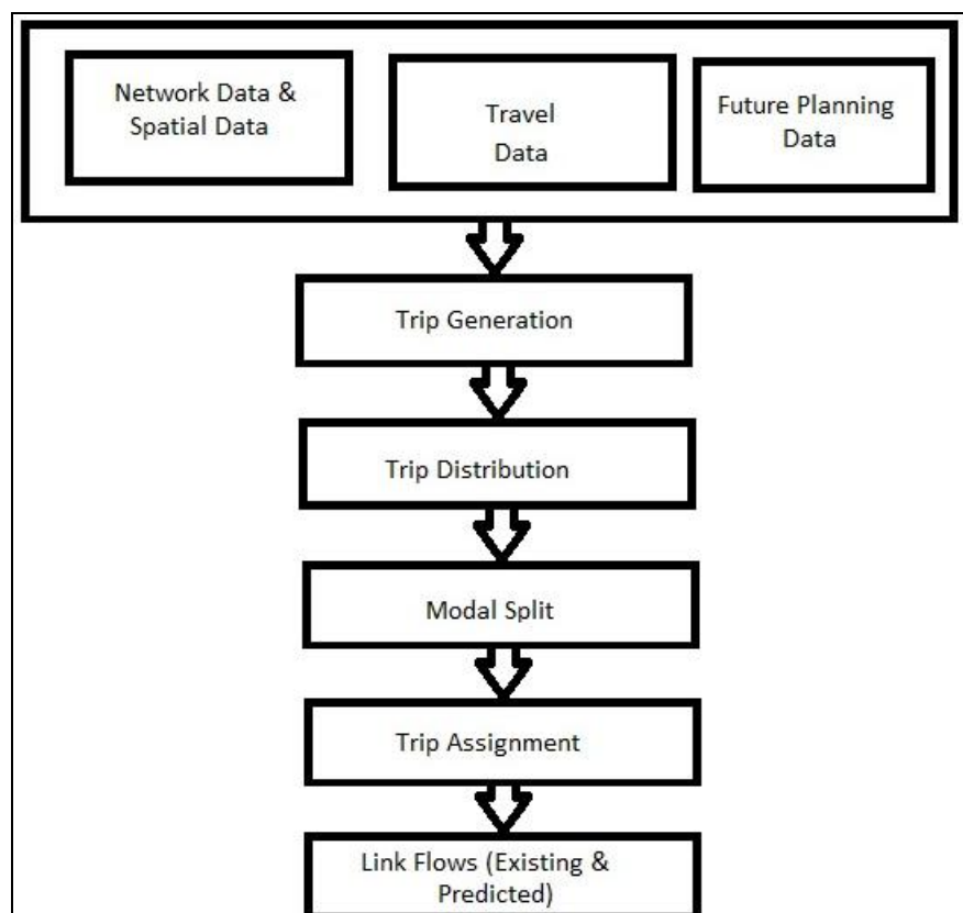
Figure 1.2: Flow of Four Stage Transport Planning Process
