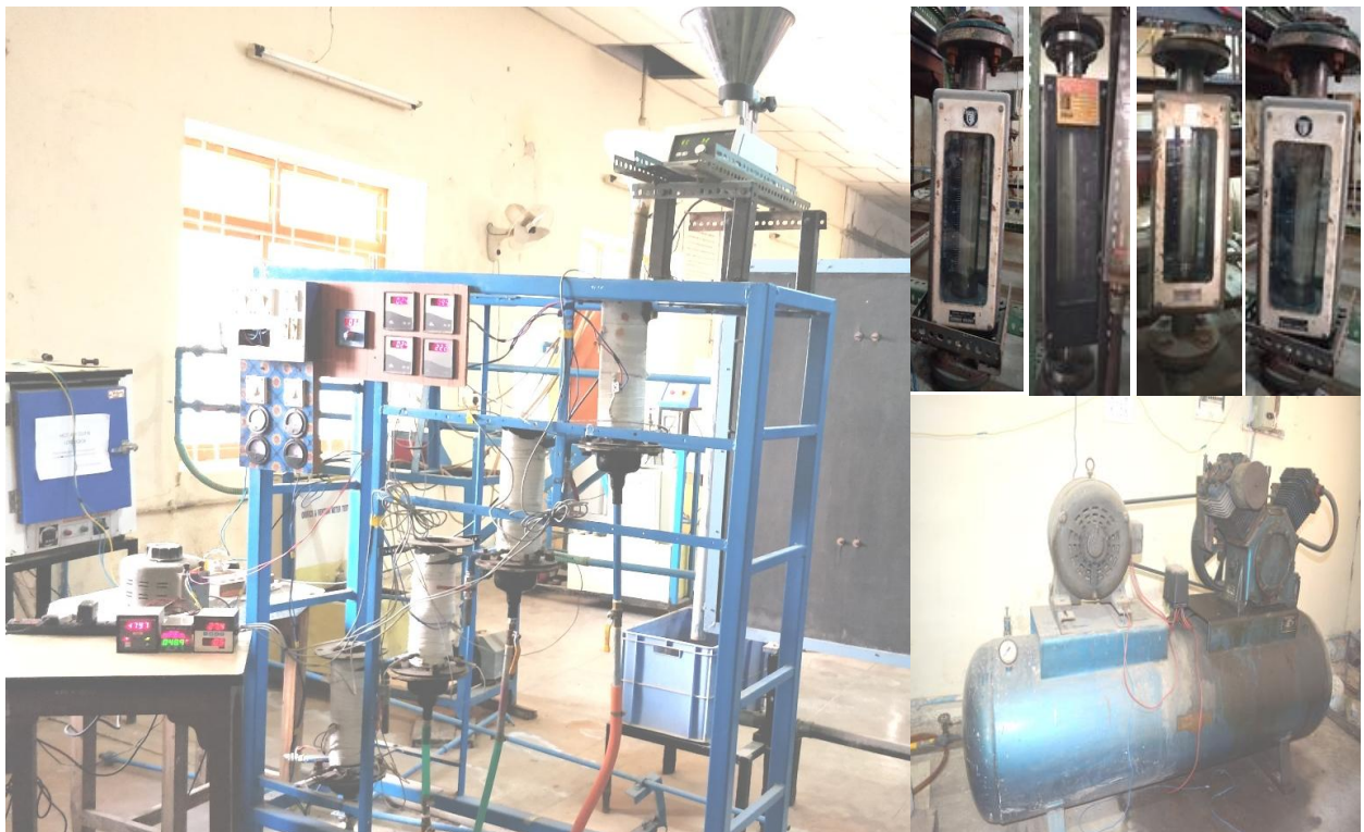
Figure 3. 4 Lab scale equipment of continuous multistage fluidized dryer
