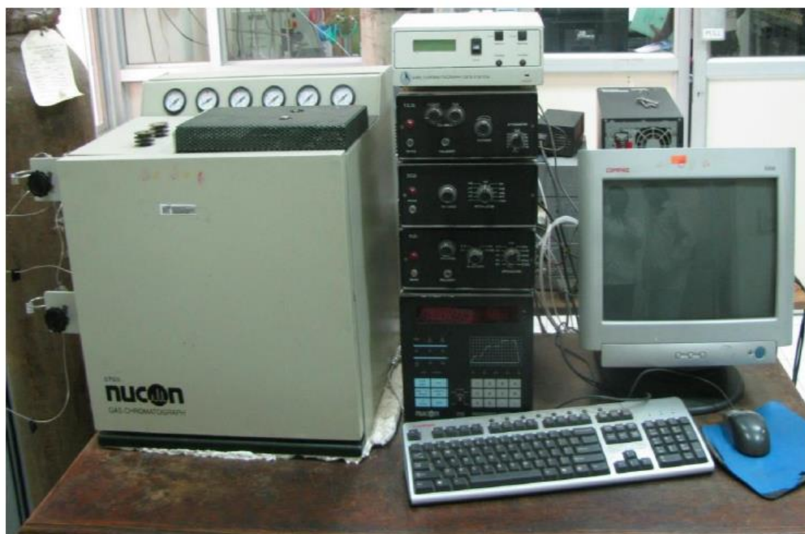
Figure.3.10. NUCON 5765 Online Gas chromatography system
