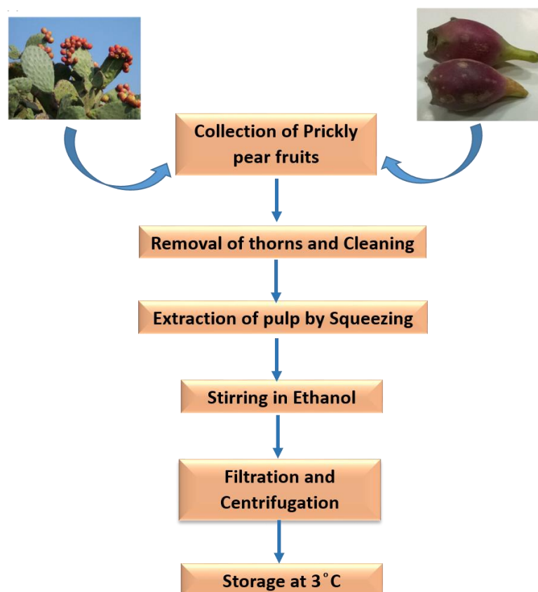
Fig. 2.4. Dye extraction process from the prickly pear fruit of cactus ( Opuntia ficus Indica ) plant.
