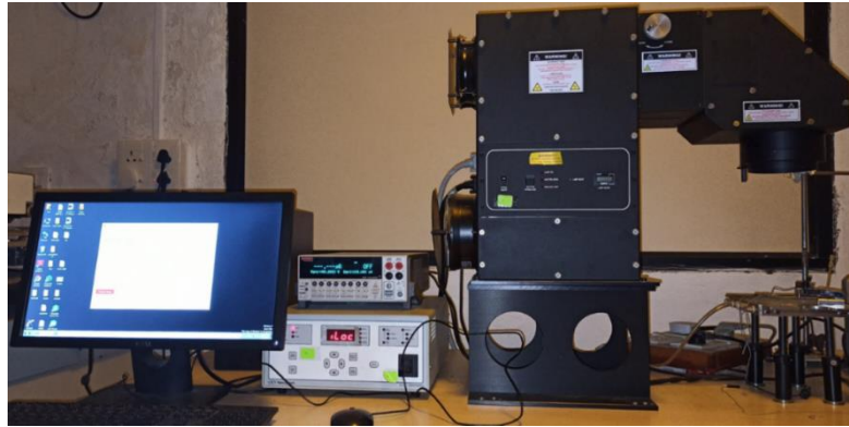
Fig. 2.16. Photograph of the solar simulator with I-V measurement set up.
