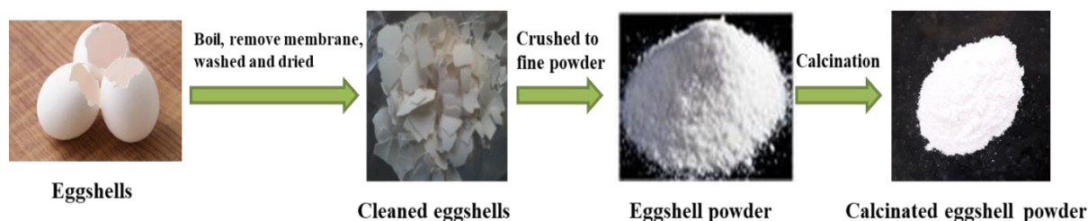
Fig. 2.2 Schematic representation of process used to convert eggshells into calcium oxide
