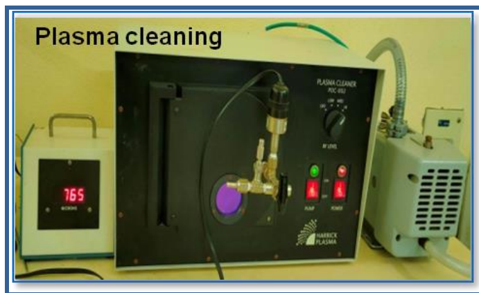
Figure 2.13 Photograph of ITO coated glass substrates during plasma treatment.
