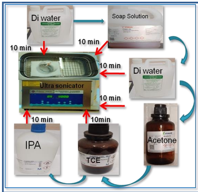
Figure 2.11. Steps involved in cleaning the patterned ITO glass substrates.
