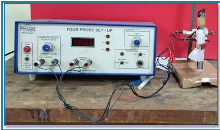
Figure 2.32 Four probe resistivity measurement setup.
