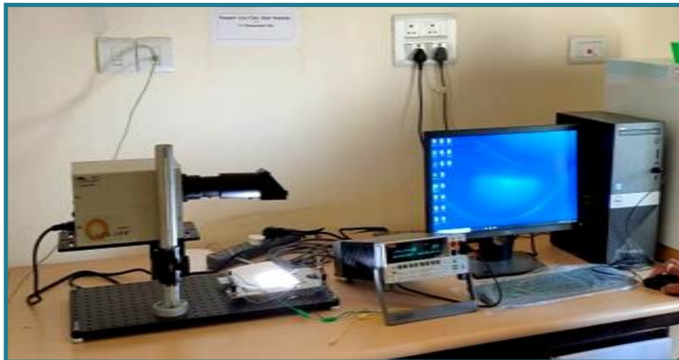
Figure 2.33 Solar simulator showing the experimental set-up for J-V characteristics of solar cell devices under illumination with Keithley 2400 source meter.
