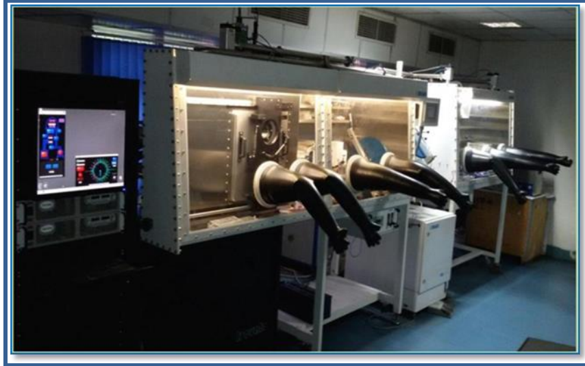
Figure 2.15 Photograph of Inert Glove Box Coating Unit used for the deposition of Ternary blends for active layer thin films.
