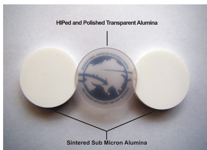
Fig. 4.10 Photograph of transparent alumina fabricated in this study (Centre), the samples at both the adjacent sides are the as-sintered alumina samples
