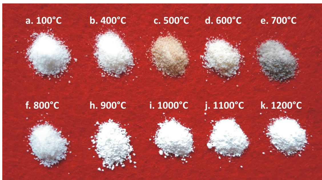
Fig. 5.5 Spinel precursor gel powders at various calcination temperatures
