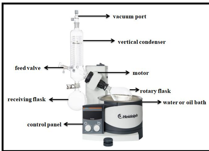
Figure 3.4: Schematic of rotary evaporator.
