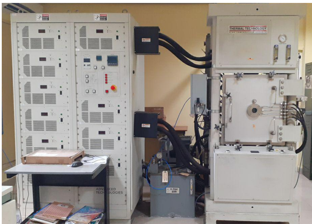
Figure 3.5 SPS set-up used for the densification of \text{ZrB}_2 -based composites.
