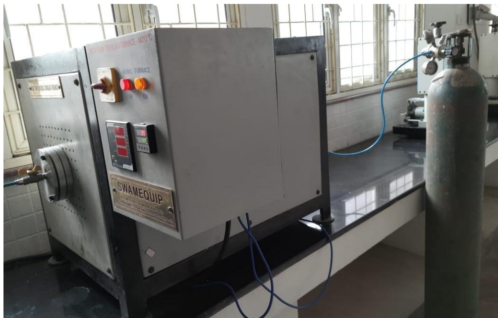
Fig. 5.6 Tubular furnace used for sintering with argon gas attachment
