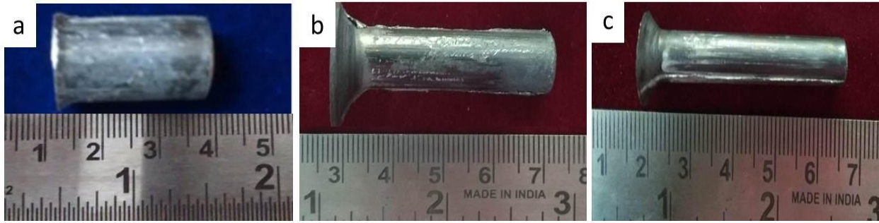
Fig. 6.16 Semi-solid extruded samples at different extrusion ratios and same die approach angle and temperature; a) 1.44, 30^\circ 550 ^\circ\text{C} , b) 2.25, 30^\circ 550 ^\circ\text{C} , c) 4, 30^\circ 550 ^\circ\text{C}
