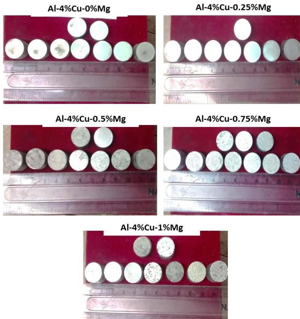
Fig. 5.7 Photographs of sintered samples at different temperatures with different compositions
