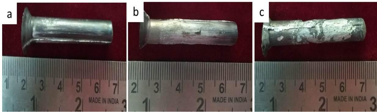
Fig. 6.11 Semi-solid extruded samples at different temperature and die with same extrusion ratio and die approach angle; a) 550 °C, 4, 30°, b) 575 °C, 4, 30° and c) 600 °C, 4, 30°
