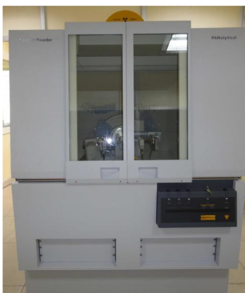
Fig. 3.16 X-ray diffractometer used for phase analysis.
