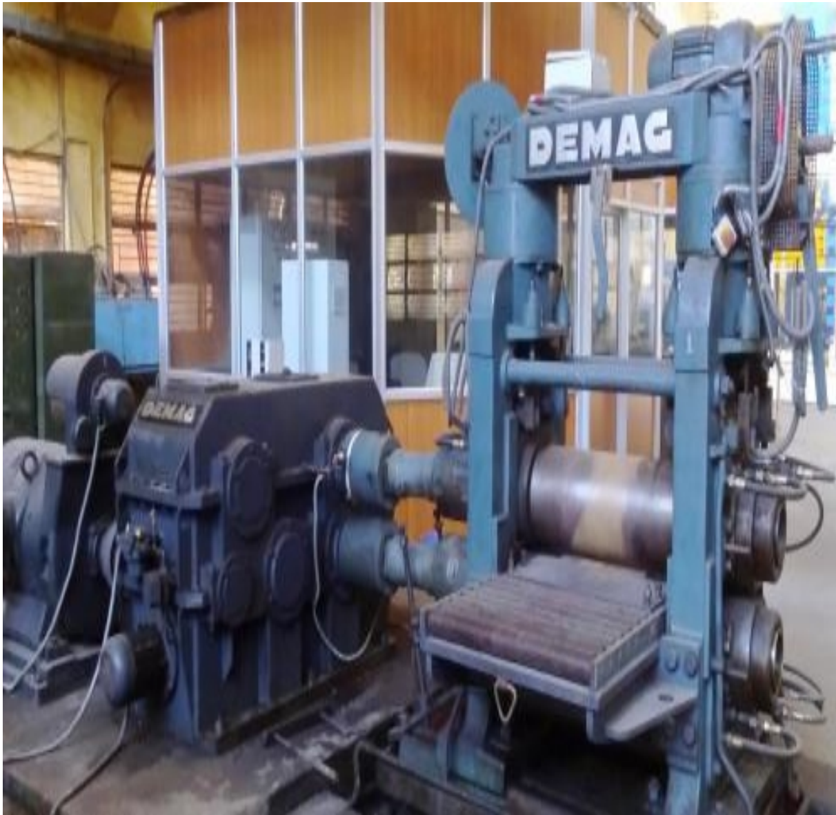
Fig. 3.7 Two high reversible DEMAG rolling mill used in the present study
