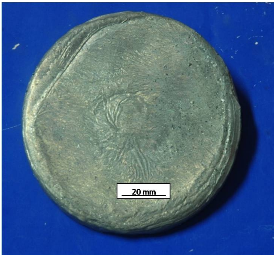
Fig. 3.3 A photograph of the pan cake melted by non-consumable vacuum arc melting process
