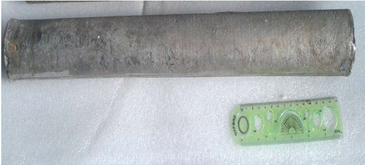
Fig. 3.5 A photograph of an ingot produced by an air induction melting process with flux cover
