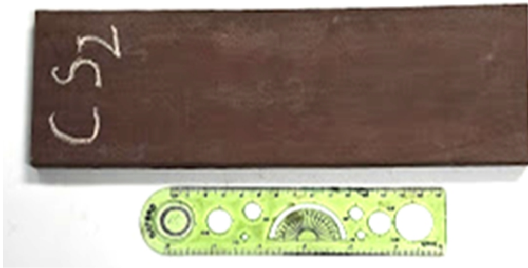
Fig. 3.8 A photograph of the hot-rolled plate from the ingot of Fe-7Al-0.35C lightweight steel.
