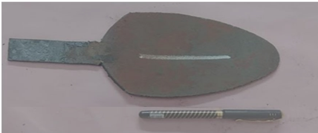
Fig. 3.9 A photograph of the hot-rolled sheet from the pancake of Fe-7Al-0.35C-1Nb lightweight steel.
