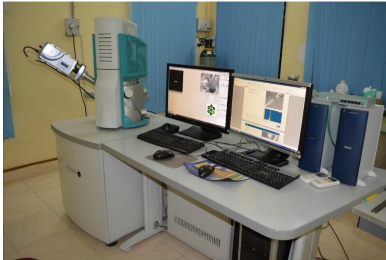
Fig. 3.1.5 TESCAN VEGA 3LMU scanning electron microscope used to observe the microstructure
