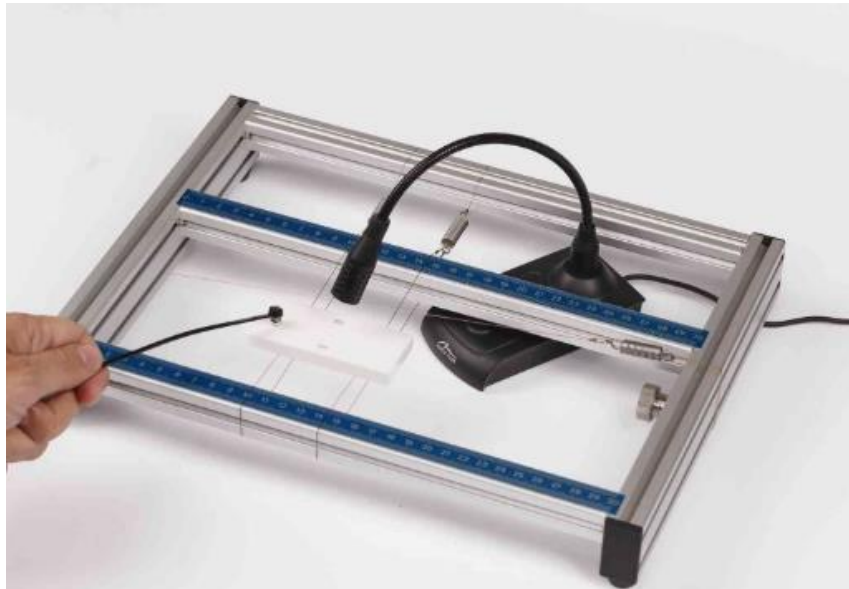
Fig. 3.1.9 RFDA basic impulse excitation technique set up as supplied by M/s. IMCE, Belgium.
