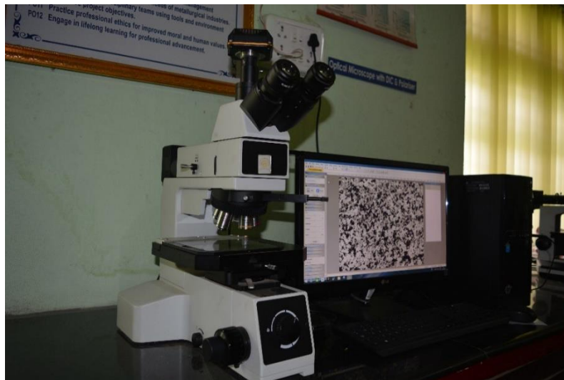
Fig. 3.1.4 Quasmo QX4RT model optical microscope used to investigate the microstructure
