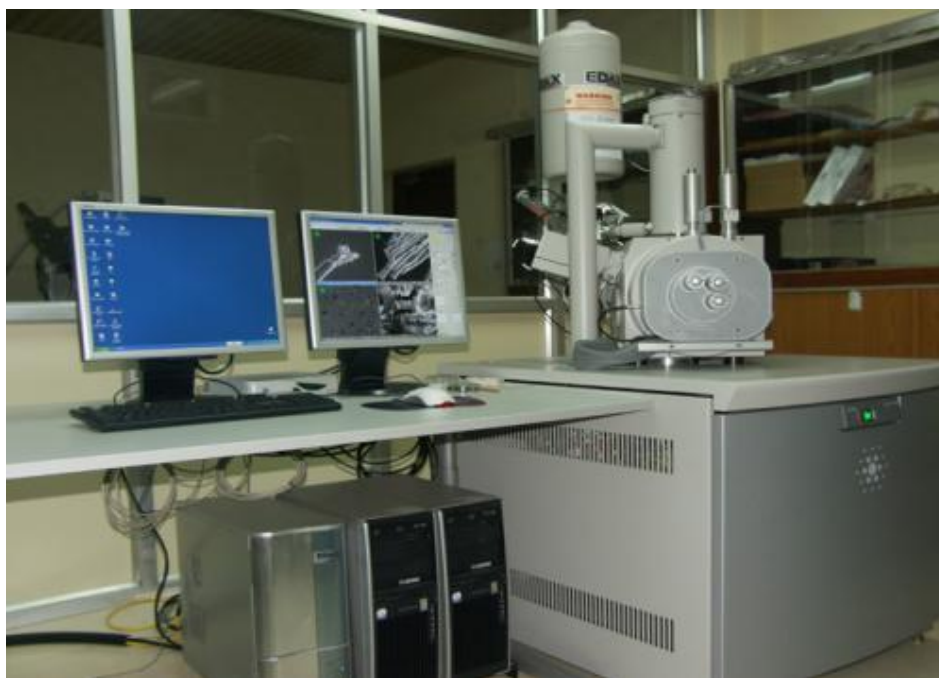
Fig. 3.4: Photograph of the Scanning electron microscope (SEM).
