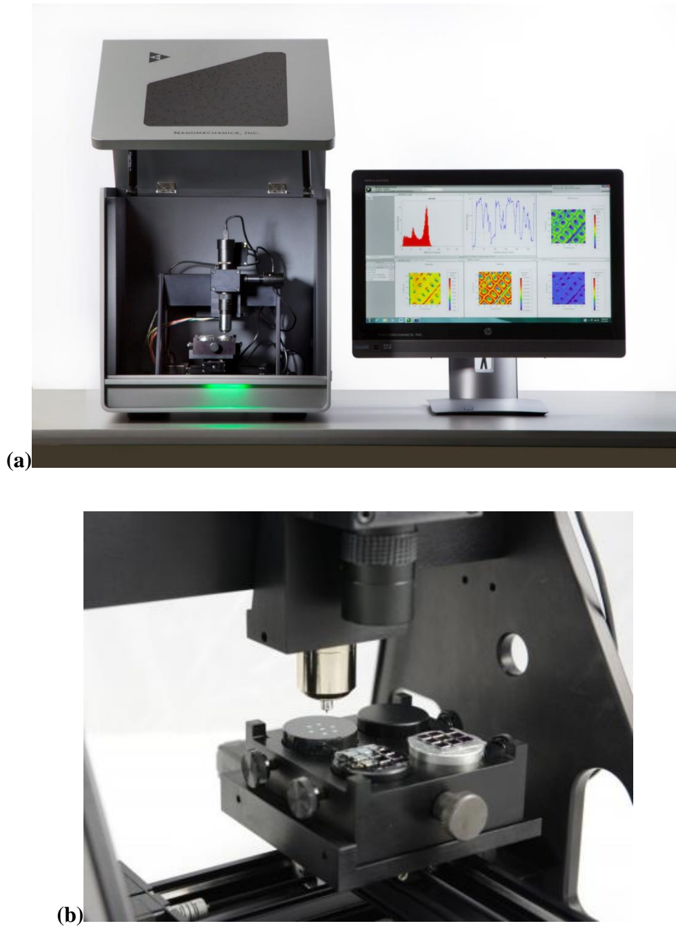
Fig. 3.9: (a) Photograph of Nano indentation equipment and (b) close view of the sample holder and indenter.
