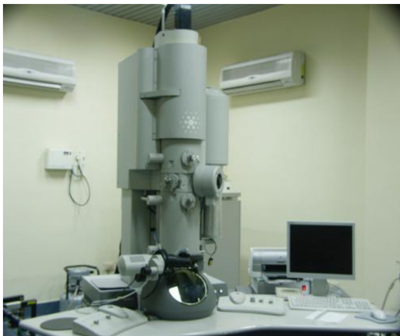
Fig. 3.6: Photograph of the Transmission electron microscopy (TEM).
