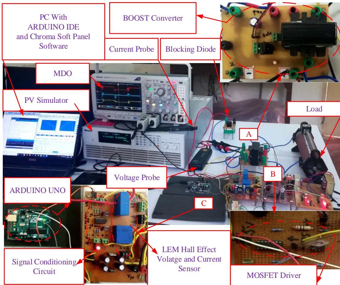
Figure 3.25: Experimental setup of the MPPT controller.
