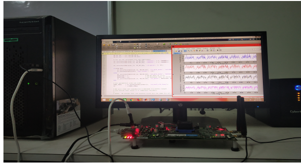
Figure 5.15: Experimental arrangement of the proposed model using WARP V3 kit.
