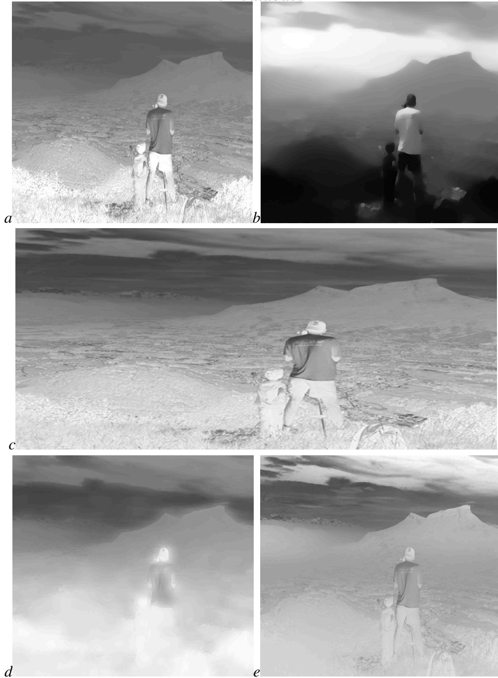
Figure 4.4: Transmission depth map of different algorithms a.Zhu et al. b. Tarel et al., c.Our Proposed d. He et al., e. Tripathi et al..
