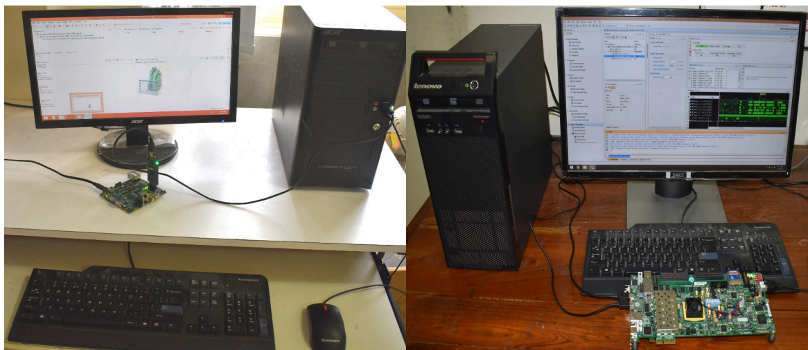
Figure 4.14: Hardware Platform Test Setup; Left: on DSP Processor TMS320C6748, Right: on Zynq 706 All programmable SoC.
