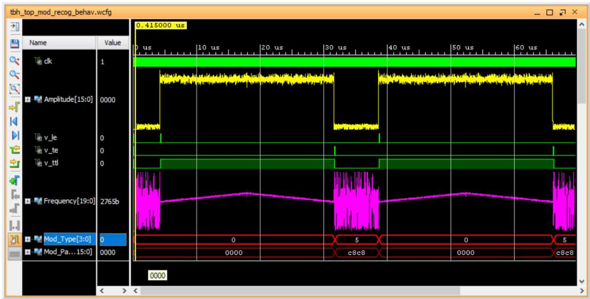
Figure 6.27: Simulation result for LFMad modulation recognition feature at 0 dB SNR.
