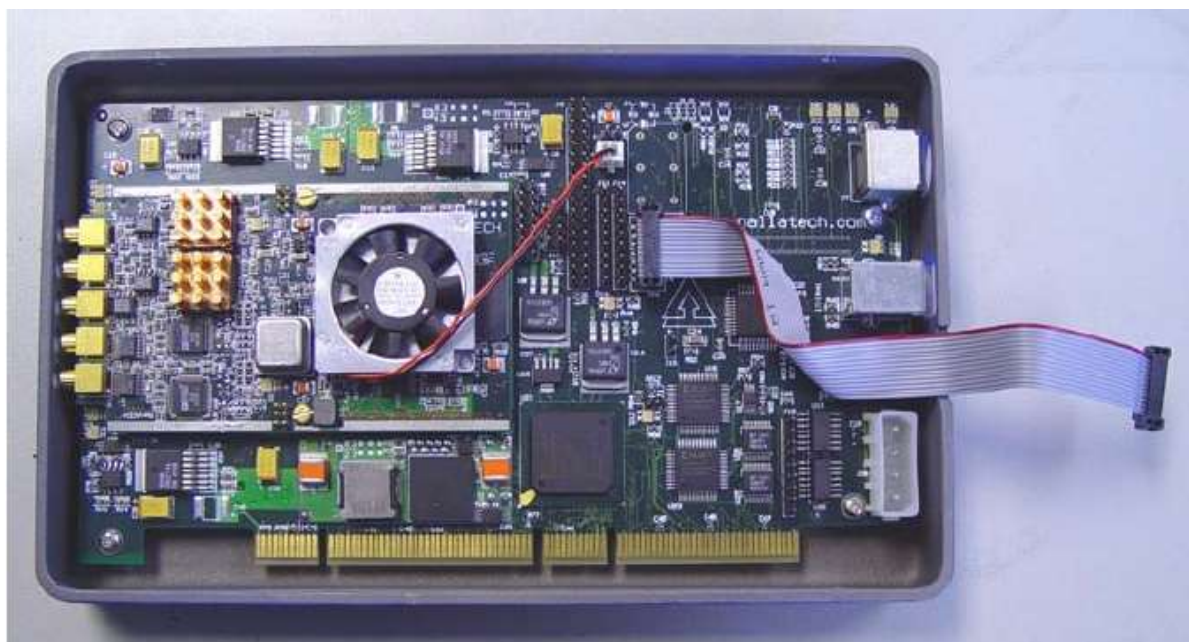
Figure 6.14: Nallatek Xilinx Virtex-4 FPGA development kit.
