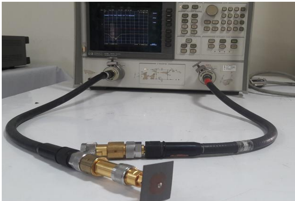
Fig.3.14 An antenna connected to one port and matched load with other port.
