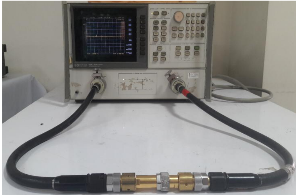
Fig.3.13 Ports are connected via a coaxial cable for matching
