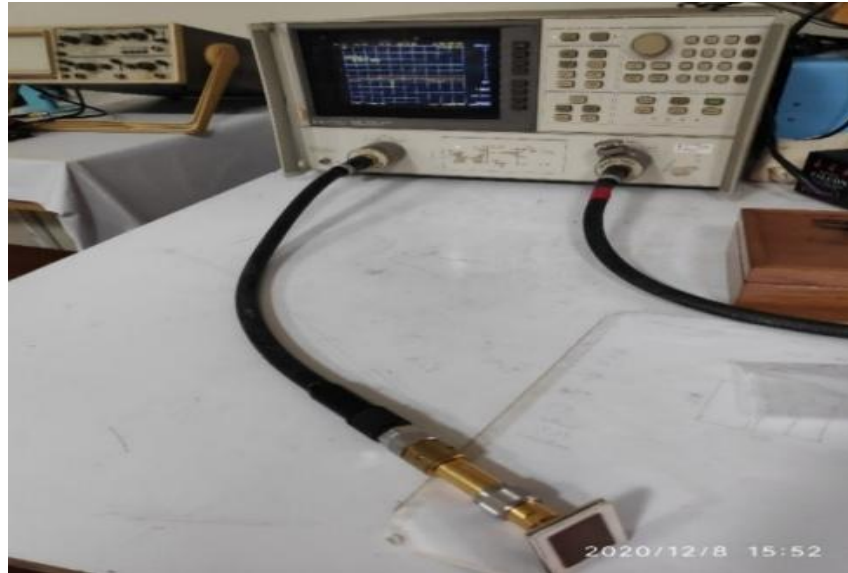
Fig.4.21. Measurement of return loss for the antenna.
