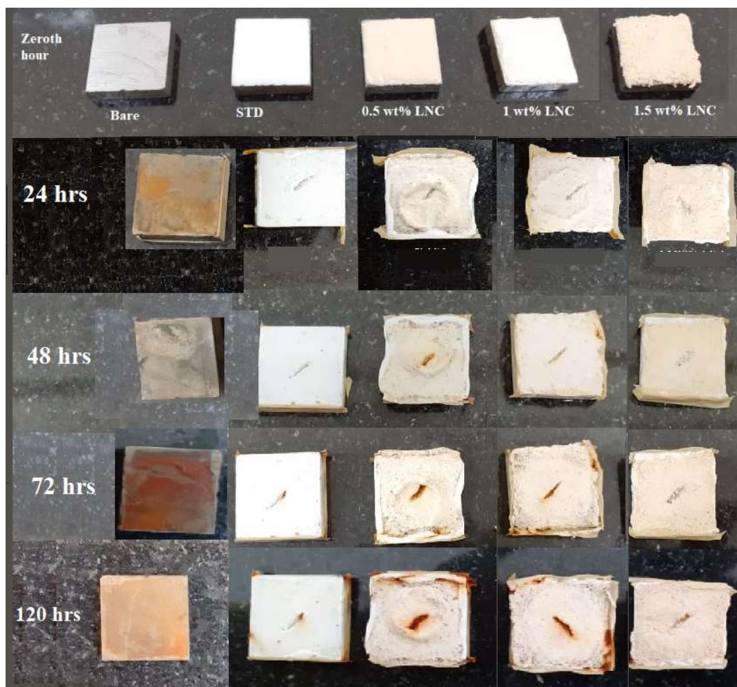
Figure 5. 18. Immersion studies (using 3.5 wt% nacl solution) of mild steel, with STD, and organic coatings (0.5, 1, 1.5 wt% lignin nanocapsules) for 120 hours.
