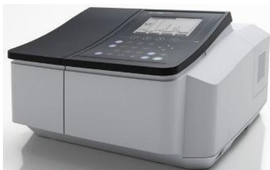
Fig. 3.8 Laboratory Ultra visible spectrophotometer (UV-1800 Shimadzu)
